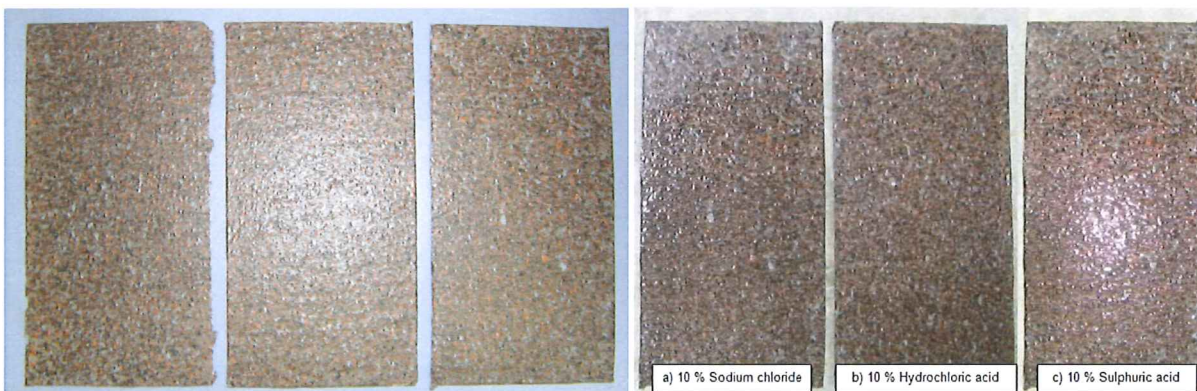
Figure 3. Chemical Resistance (Left: before immersion, Right: after immersion)
